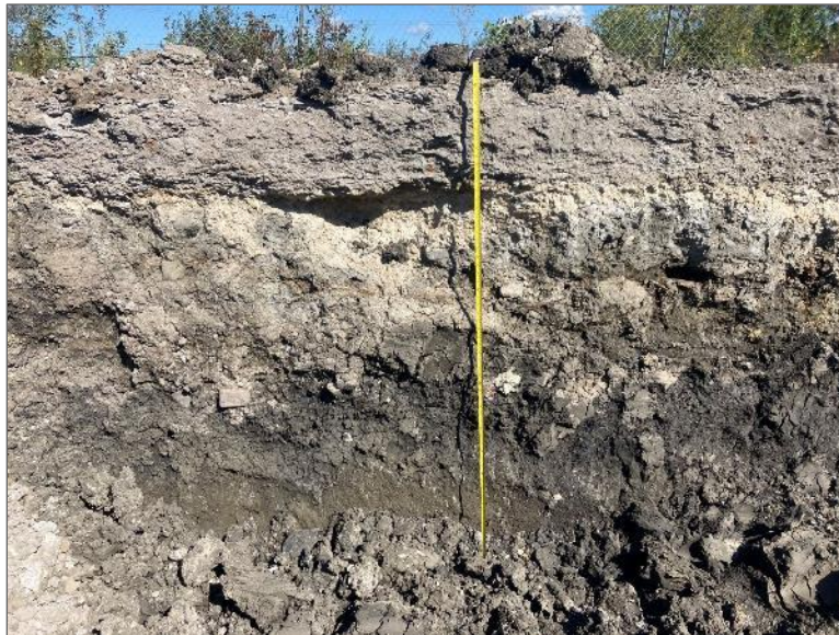
Photo 4 – Soil stratigraphy at Excavation 1 extending to 1.5 metre below ground surface.
