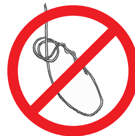
Figure 2 - Prohibited Traditional Double-loop Knot
