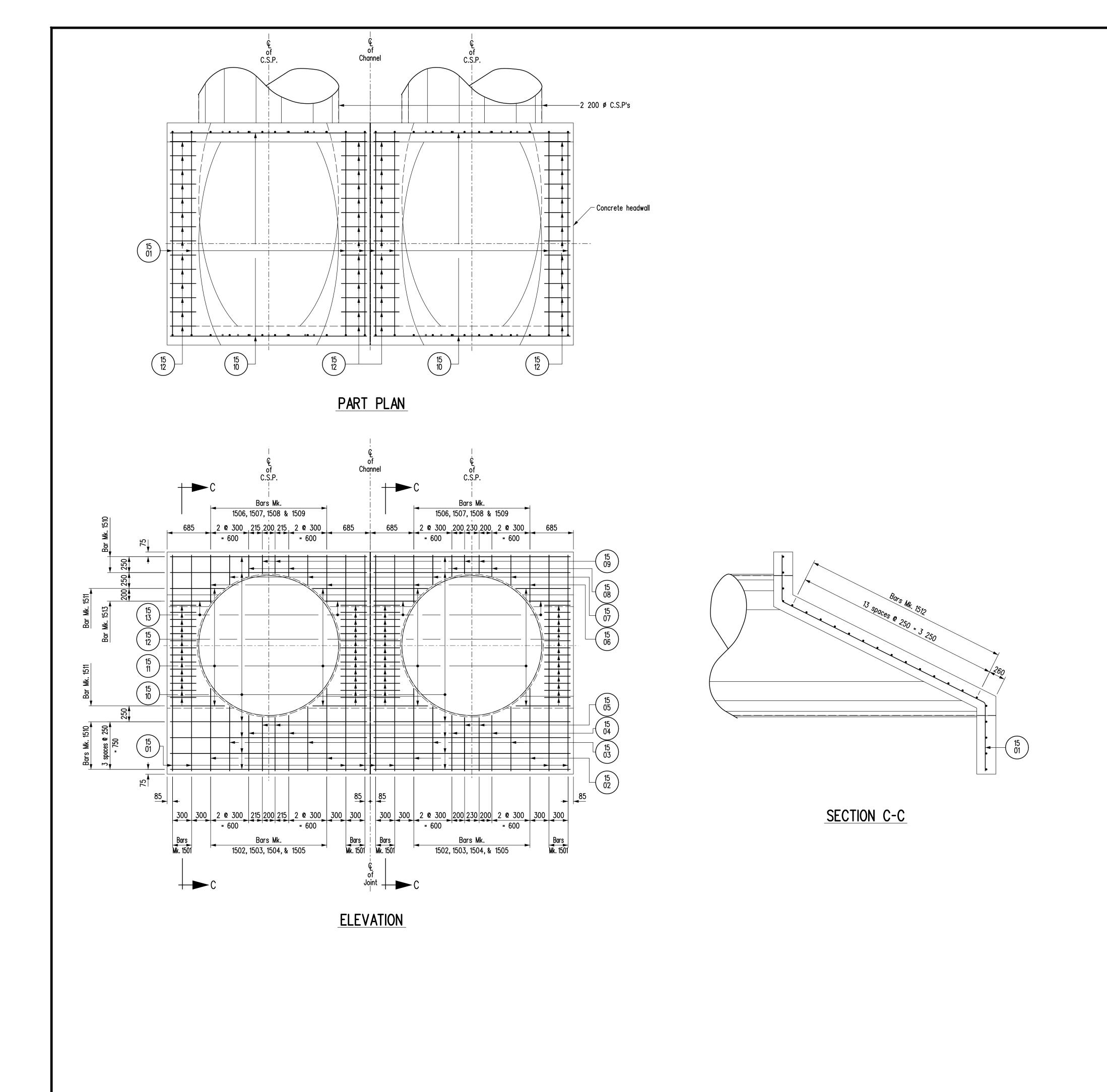
BILL OF REINFORCING STEEL FOR 2 REINFORCED CONCRETE HEADWALLS PIN DIAMETER TYPE LENGTH BENDING DIAGRAM BENT 5 400 135.65 1 590 730 1502 STR 1 300 8 16.33 1503 STR 12.69 1 010 1504 STR 880 11.05 1505 STR 840 8 10.55 1506 STR 750 8 9.42 1507 STR 460 8 5.78 1508 330 STR 8 4.14 1509 STR 290 3.64 8 1510 STR 3 090 24 116.43 1511 STR 850 16 21.35 1512 STR 410 112 72.09 1513 STR 650 8.16 8 Total mass of reinforcing steel 427.28 kg
