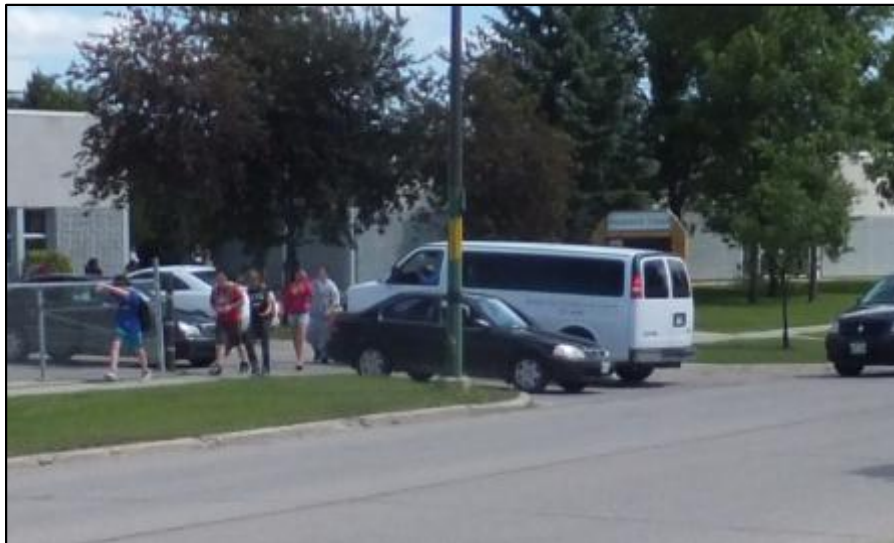
This school's driveway throat is very short, and vehicles queued to leave prevent vehicles entering from turning into the loading area, causing queuing onto the street. Also, students leaving the school are weaving between queued cars.
