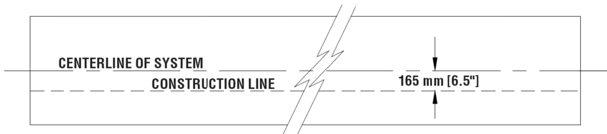
Figure 48 (Top view of concrete foundation)
