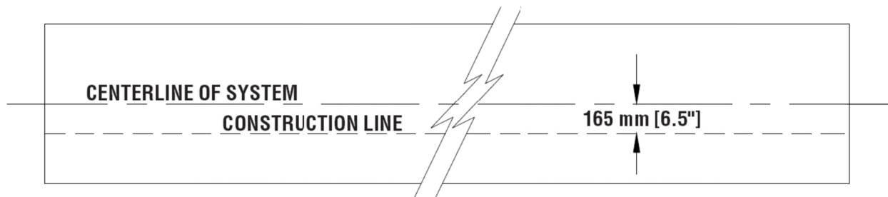
Figure 16 (Top view of concrete foundation)
