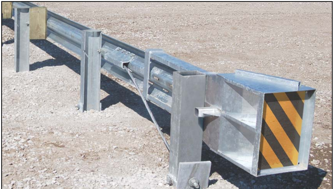
Figure 5. View of FLEAT-SP Steel End Post #1
