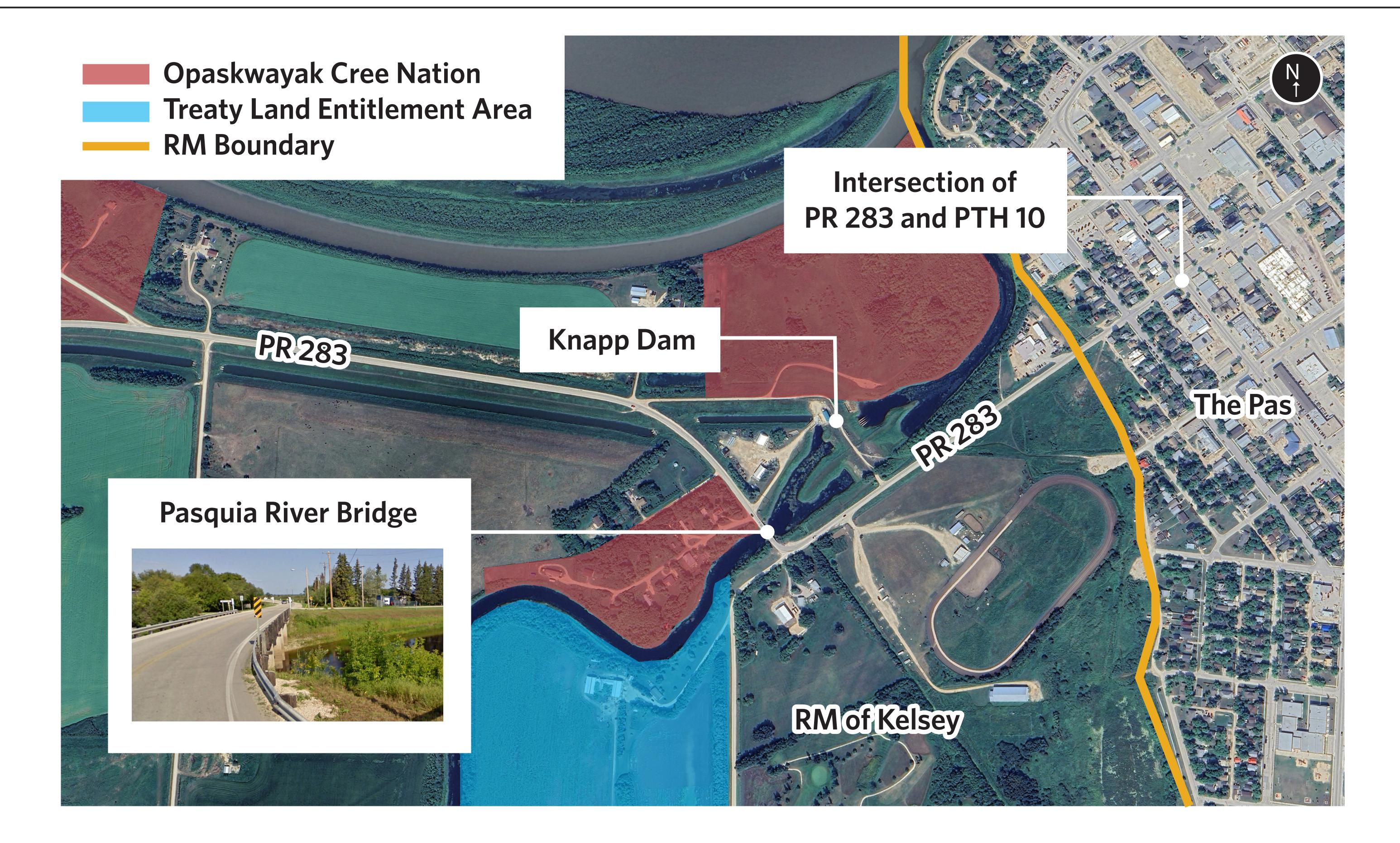
MTI engaged WSP to complete a Functional Design Study of PR 283 and a Preliminary Design Study of a new bridge over the Pasquia River (including realignment of PR 283).
