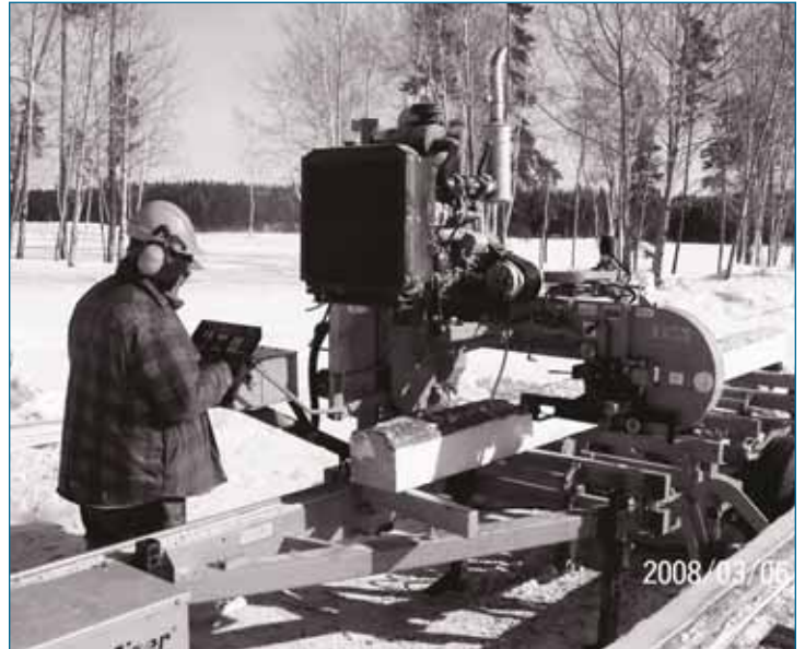
Frontiers Foundation encourages harvesting local trees and making timber for housing construction using a portable sawmill that can be towed where it is needed.
