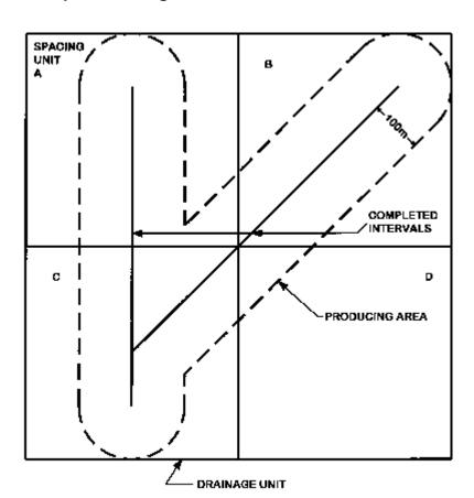
**DETERMINATION OF PRODUCING AREA Example: Single-Leg Horizontal Well**
