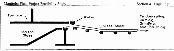
Figure 4. Simplified plate glass forming process.
