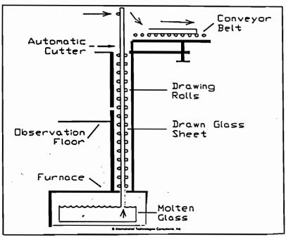
Figure 3. Simplified vertical draw sheet process.
