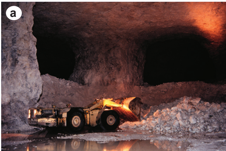
Figure 6: Underground photos at the Tanco mine (with permission of Sinomine): a) scooptram close to one of the spodumene zone pillars illustrating the room and pillar method used at Tanco; b) custom designed aerial lifts.
