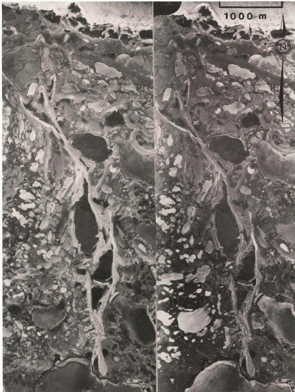
FIGURE 13. Stereopair (A22955-12, 13) showing abandoned beach deposits south of Gordon Point. Shoreline of Hudson Bay at top of photographs. Numerous swamps on both sides of the beach ridge restrict access to the deposit.
