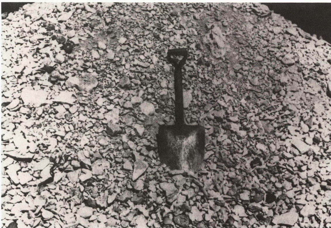
FIGURE 11. Cobbly coarse pebble gravel of deposit 32042, ground observation site C6. Shovel 1.0 m high. Lithology is predominantly limestone with minor Precambrian crystallines.
