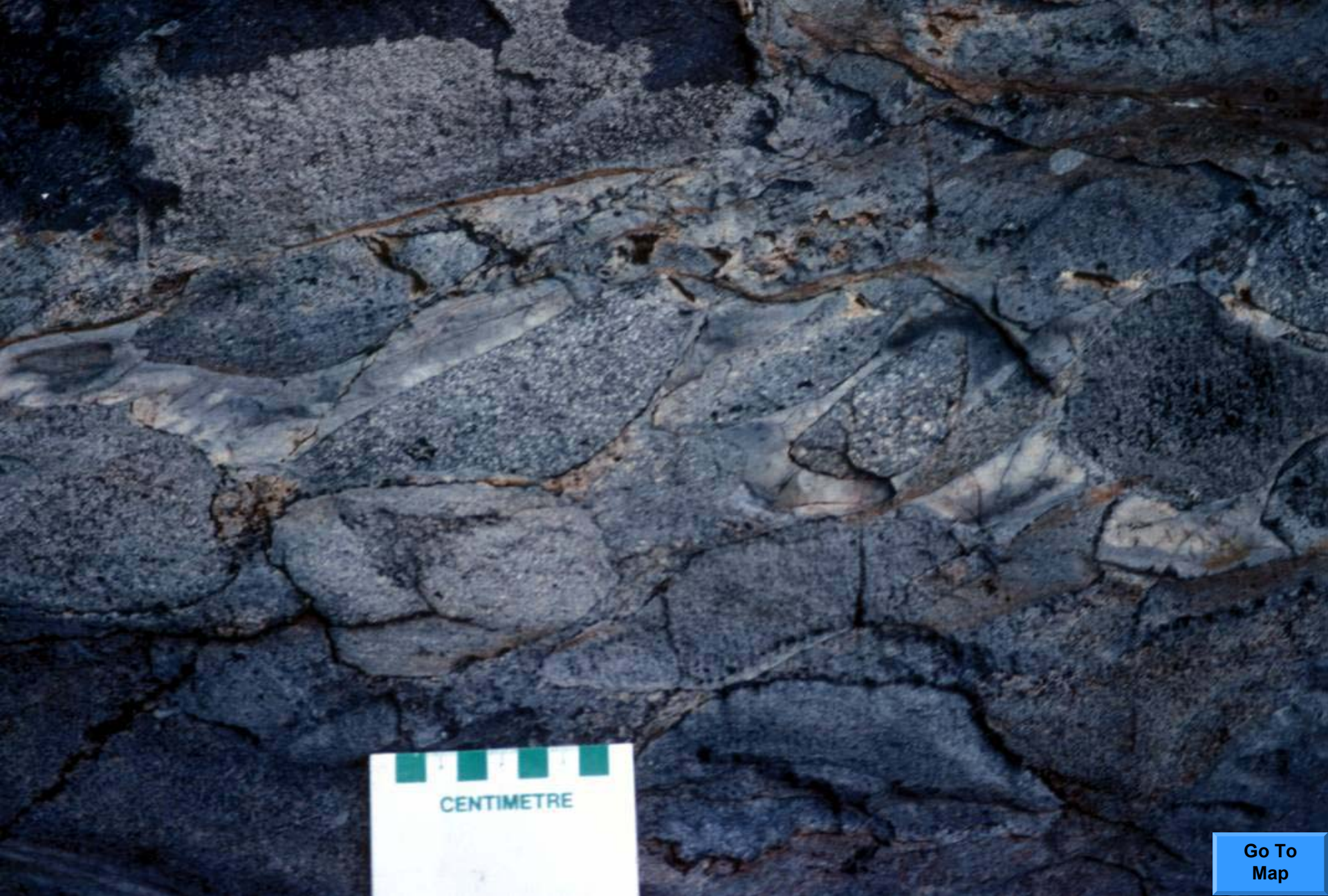
Figure 22: Framework-supported, heterolithic, intermediate to felsic cobble- to boulder-conglomerate (unit S4a). This unit occurs as screens between massive rhyodacite, along the shoreline and to the east in the area north of Stuart Lake. UTM Zone 14U, 449652E, 6067009N.
