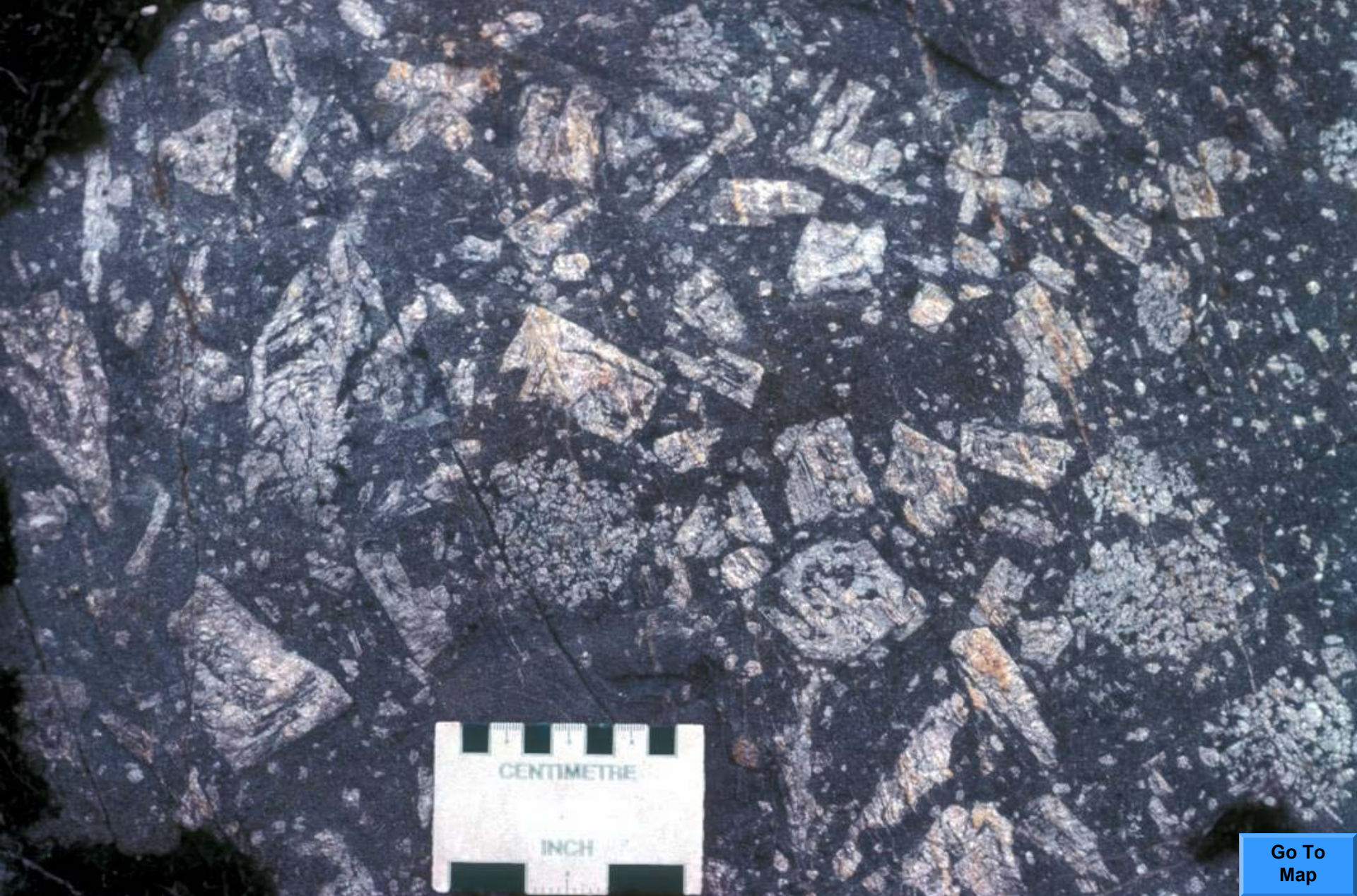
Figure 32: Megaphyric, cumulophyric diabase (unit L1e). Note that large plagioclase phenocrysts locally display synneusis texture and are partially resorbed, whereas smaller plagioclases are aggregated in round cumulophyric bodies, one of which (at lower right) is partly dislocated. The diabase also contains 2–5 mm pyroxene phenocrysts altered to hornblende. UTM Zone 14U, 441521E, 6061775N.
