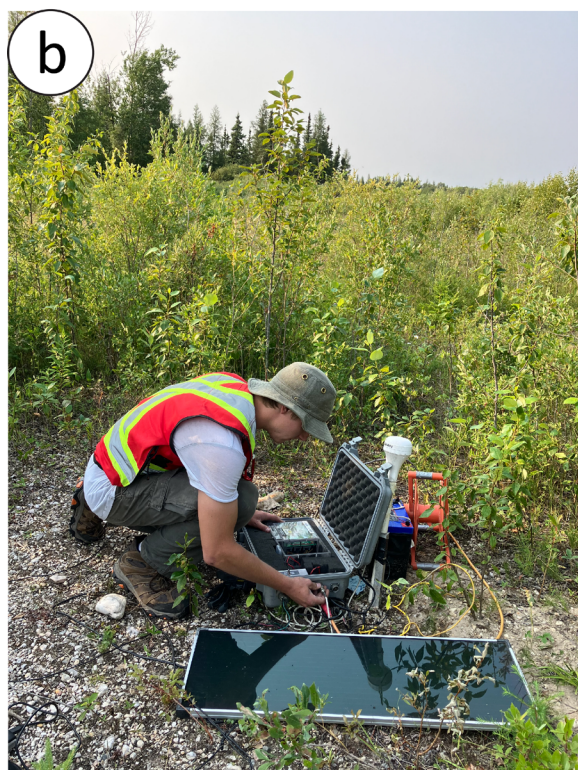
Figure GS2024-17-2: a) Layout of a long-period magnetotelluric (LMT) station. Installation only requires digging 4–6 temporary holes in the ground to a depth of 30–40 cm. The station typically occupies an area that is up to 100 by 100 m in size; b, c) Examples of a LMT system (Narod Geophysics Ltd.’s Narod Intelligent Magnetotelluric System [NIMS]) being deployed in the field in Manitoba.
