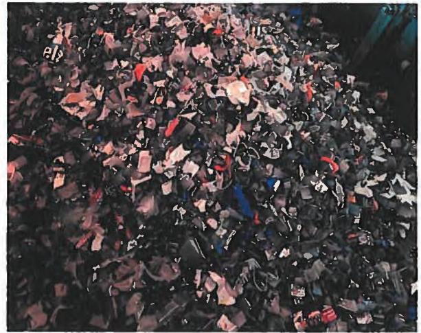
Containers in Bags Grinded for Feedstock to the ROC
