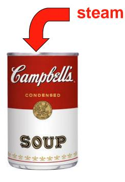
Heat has to diffuse inwards to coldest point in the can
