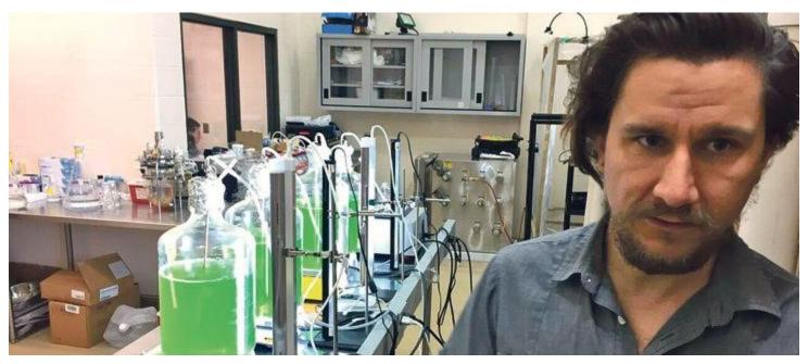
University of Manitoba researcher Ryan Sestric is testing a system where synthetic fish waste is the primary feed source for specialized algae, which can then be harvested for a variety of uses. | Ed White photo
