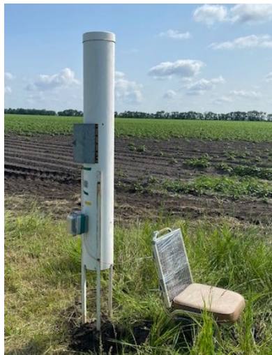
Fig.8 (left). Spornado passive spore trap set near potato field. Photo: Vikram Bisht, (Manitoba Agriculture).
